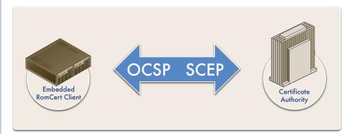
RomCert is a platform independent implementation of the Online Certificate Status Protocol (OCSP) and the Simple Certificate Enrollment Protocol (SCEP) and makes embedding security certificate management into resource sensitive embedded systems and consumer electronics fast, easy and reliable, while decreasing time to market.
